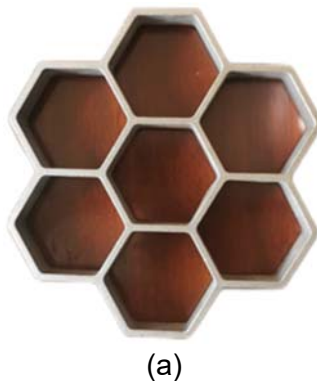
Fig.1 The honeycomb compound anti-wear device in the furnace
